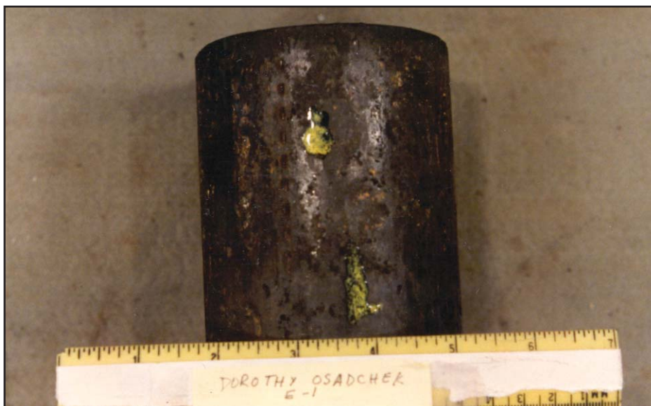
Figure III-2: Example of H_2S Attack
