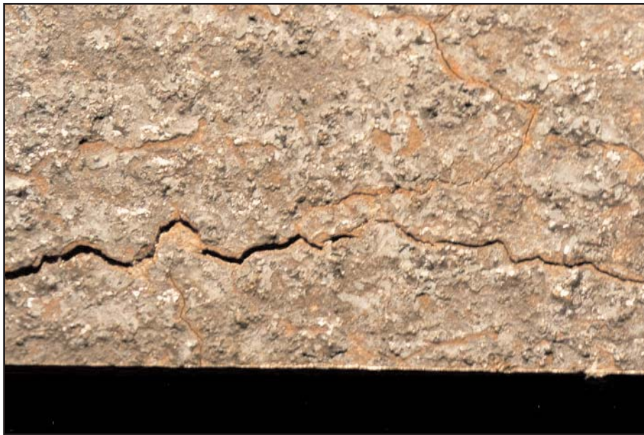
Figure IX-14: Cracks on Internal Surface Covered with Iron Oxide Corrosion Products
