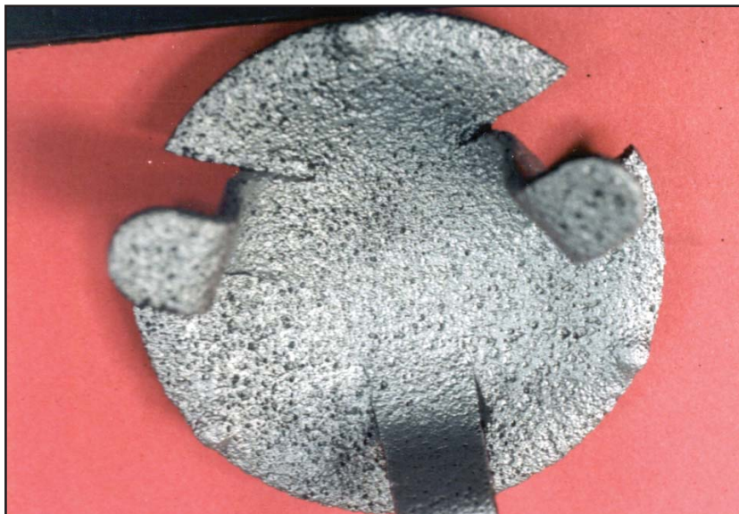
Figure V-4: Close-up of Pitting Corrosion
