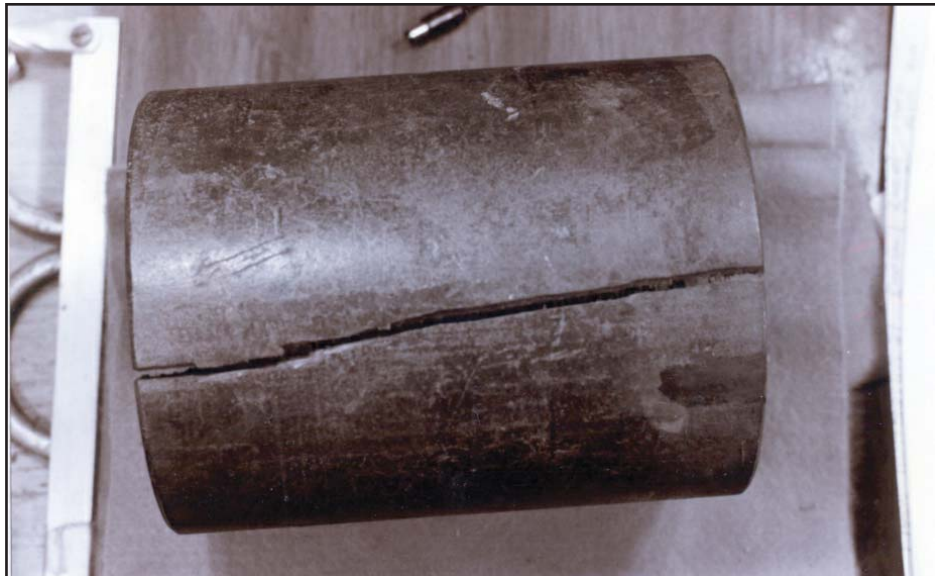
Figure III-11: Sulfide Stress Cracking of a Casing Collar
