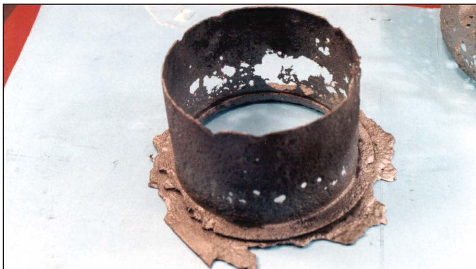
Figure V-8: Ammonium Chloride Corrosion on SS410 Trays
