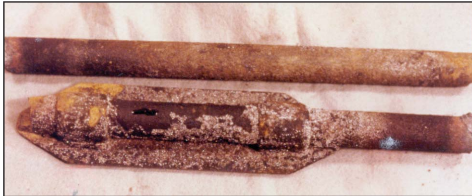
Figure III-4: H 2 S Attack on Sucker Rods
