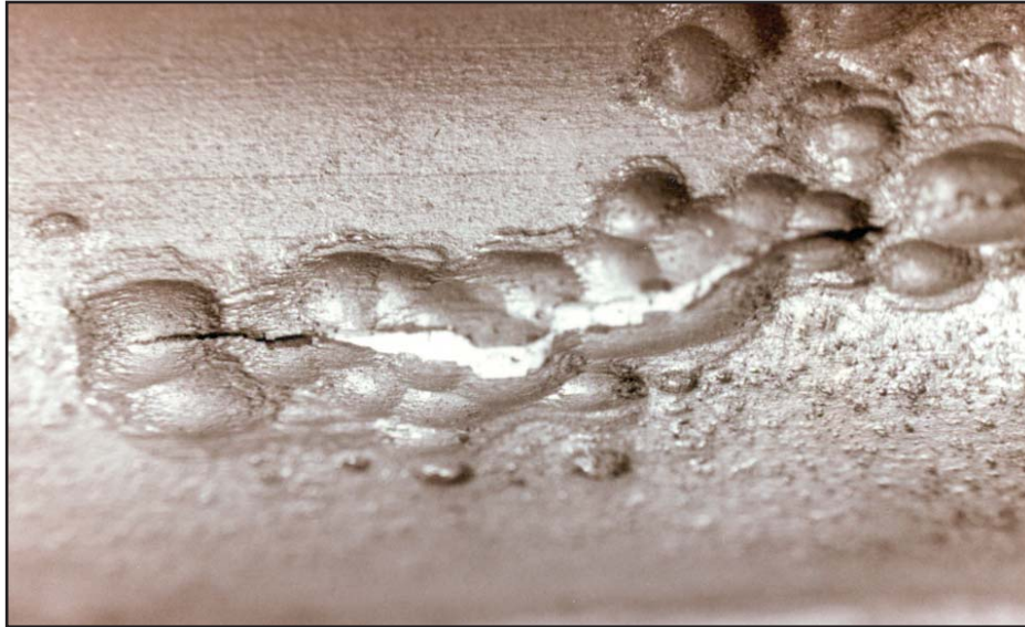
Figure I-15: Close-up Tubing with Wormhole Attack
