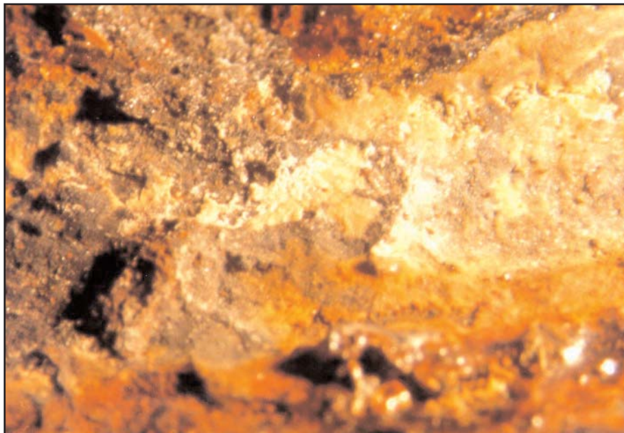
Figure IX-41: Iron Oxide Layers and Tubercles Overlaid with Water-formed Deposit Layers
