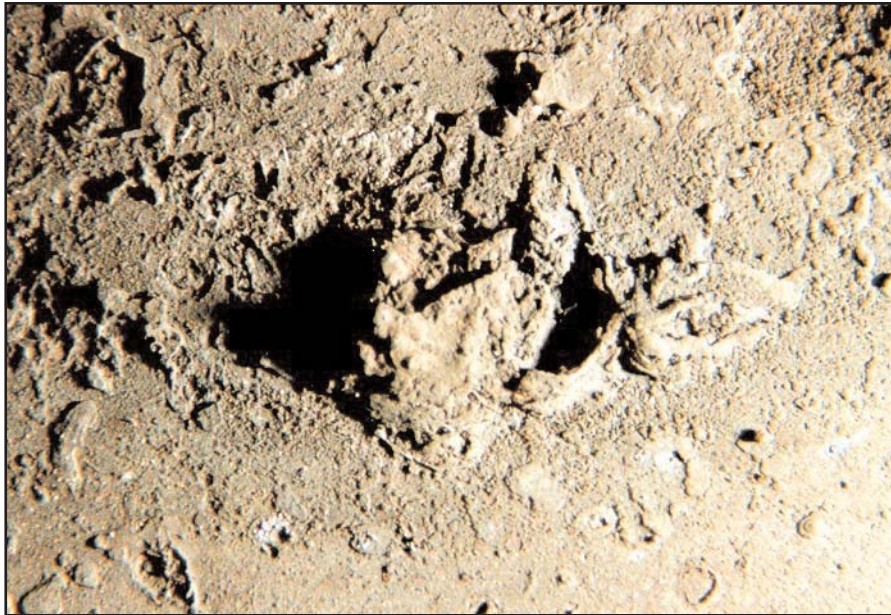
Figure IX-6: Iron Oxide Tubercle with No Flow Orientation
