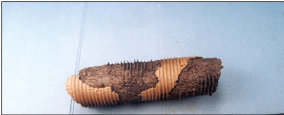
Figure VII-2: Close-up of De-alloying Tubes — H 2 S Corrosion 90-10 Cu:Ni Heat Exchanger Tubes
