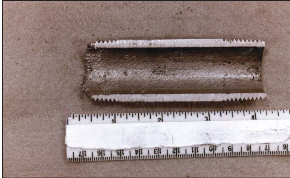
Figure I-45: Flow-Enhanced Corrosion at Nipple Joints
