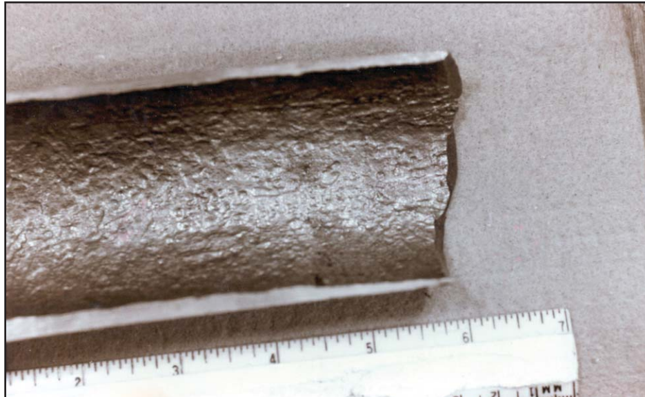
Figure I-19: Parted Tubing by Ringworm Attack
