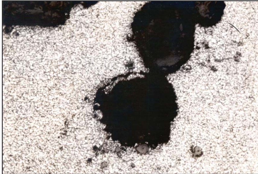
Figure VIII-17: Fuel Storage Tank Corrosion
