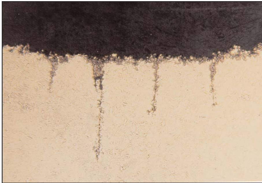
Figure IX-37: Corrosion Fatigue Fissures Penetrating from Base of Depression
