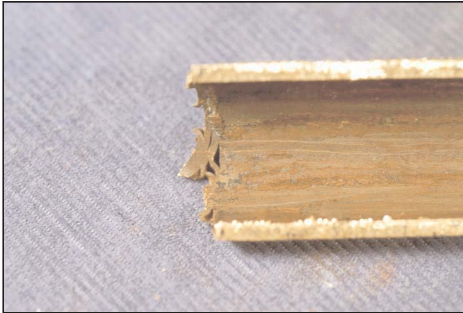
Figure IX-30: Numerous Transversely Oriented Fissures near Fracture Edge
