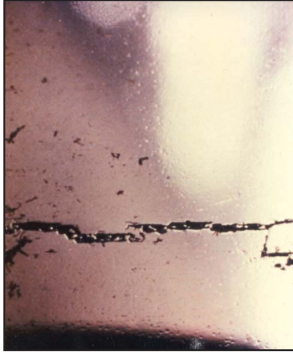
Figure III-13: Chloride Stress Corrosion in Stainless Steel
