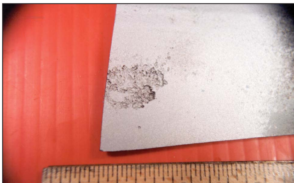
Figure VIII-16: Fuel Storage Tank Corrosion
