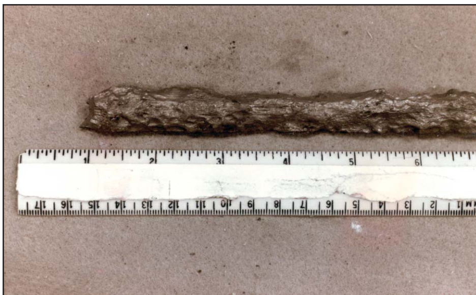
Figure II-6: Areas of Metal Loss on Sucker Rods
