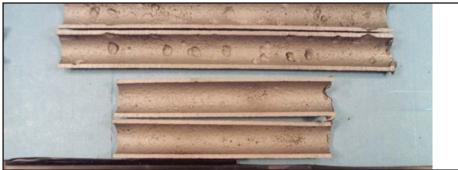
Figure VIII-7: Oxygen, H_2S , and CO_2 Corrosion
