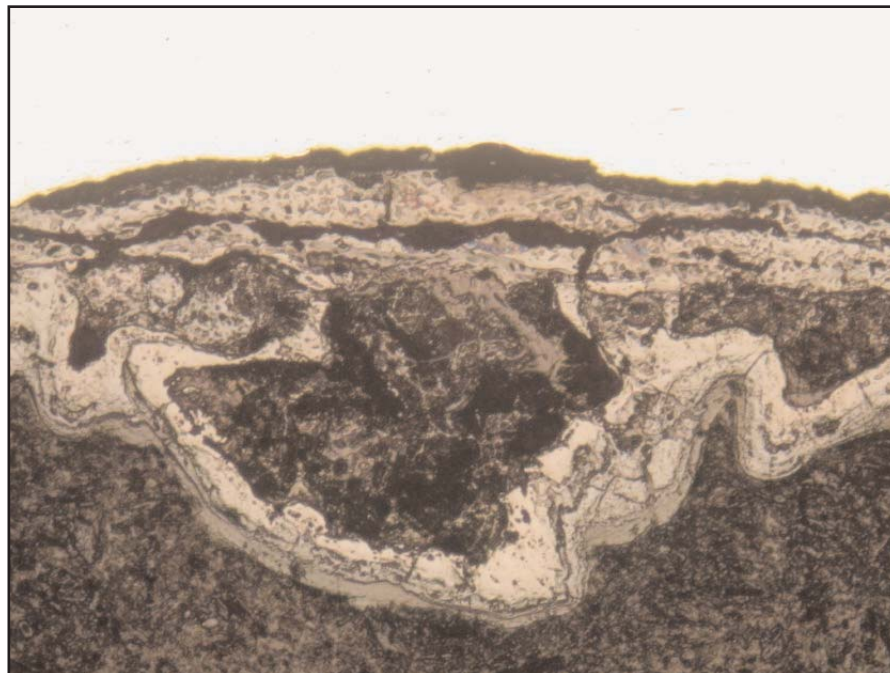
Figure IX-43: Metallographic Cross-section of Rough-surfaced, Undercut Depressions beneath Hollow Iron Oxide Tubercle
