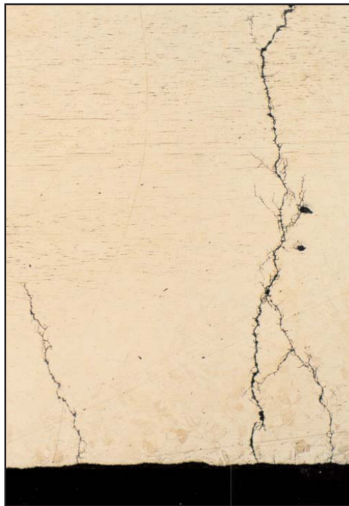
Figure IX-16: Metallographic Cross-section Revealing Branched, Transgranular Cracks Penetrating Outward from Internal Surface
