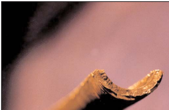
Figure IX-27: Wall of Admiralty Brass Heat Exchanger Tube Penetrated by a Crack
