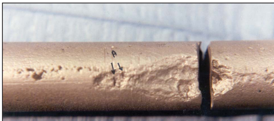
Figure III-6: Sulfide Stress Cracking
