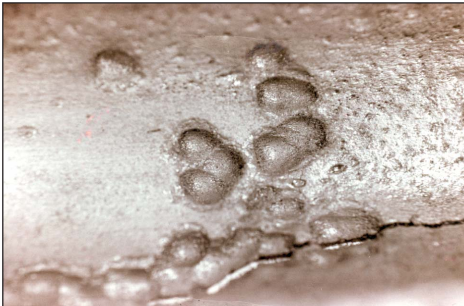
Figure I-16: Wormhole Effect — Cluster of Large Pits
