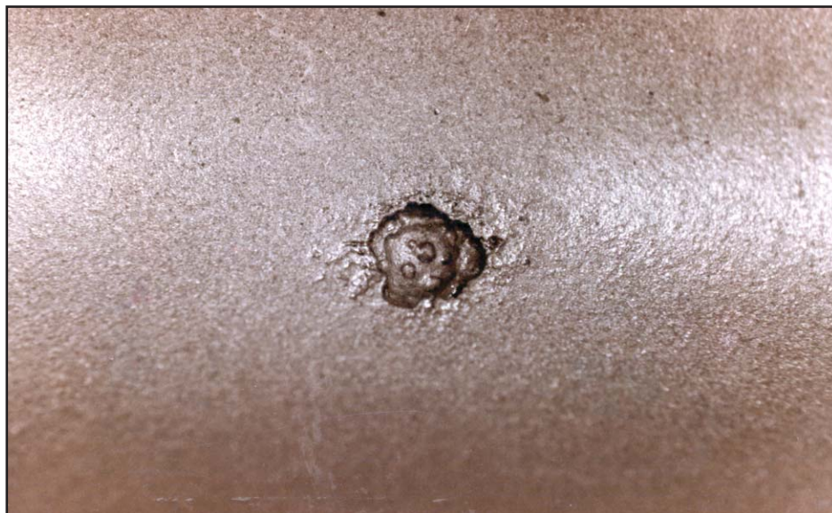
Figure IV-4: The Terraced Effect
