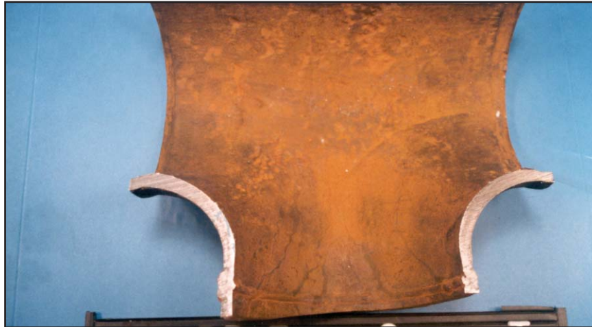
Figure VIII-1: Erosion Corrosion — Carbon Steel Tee
