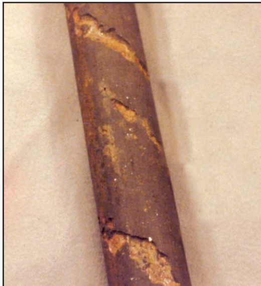
Figure I-26: Corrosion Resulting from Rolled-in Inclusions
