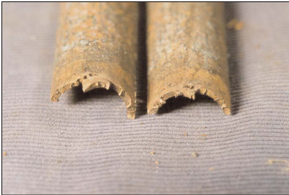
Figure IX-29: Brittle Fracture Edge Containing Multiple Crack Initiation Sites
