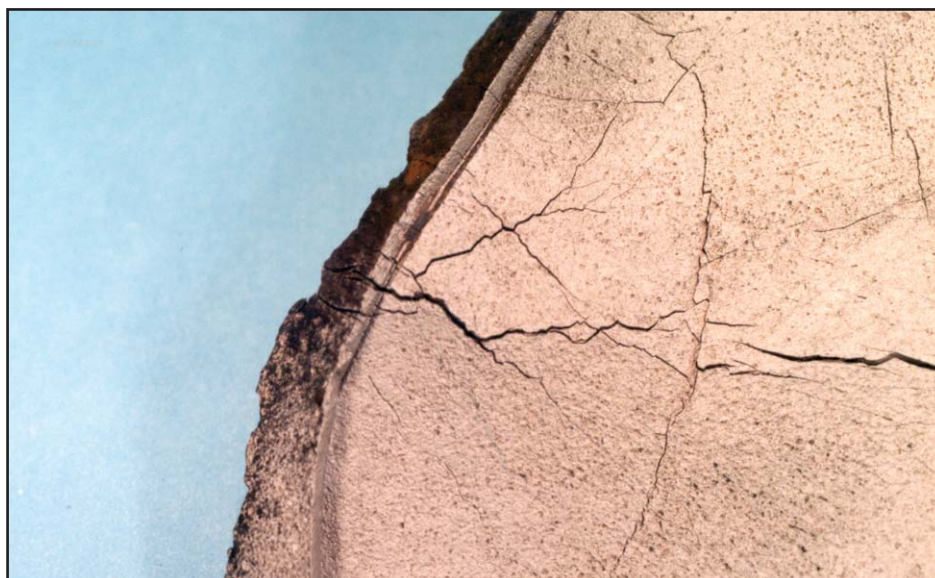
Figure V-10: Stress Corrosion Cracking Failure
