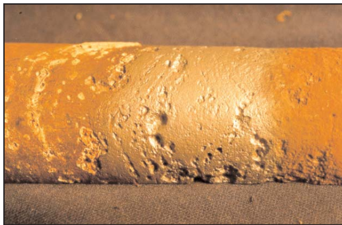
Figure IX-24: Deposits Removed to Reveal Depressions
