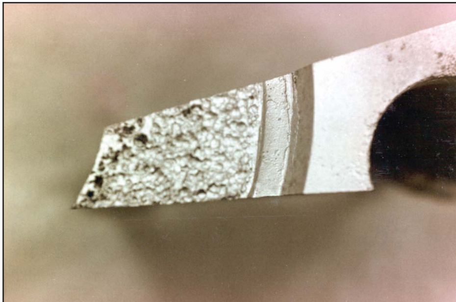
Figure I-6: CO 2 Attack — Honeycomb Pattern
