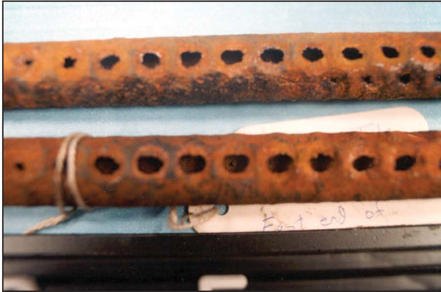
Figure VIII-3: Erosion-Corrosion — Carbon Steel Overhead Exchanger Tubes
