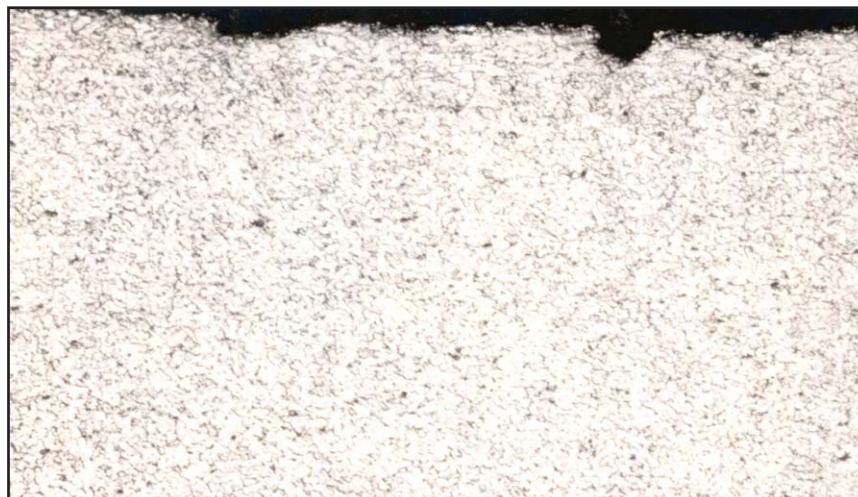
Figure VIII-18: Fuel Storage Tank Corrosion
