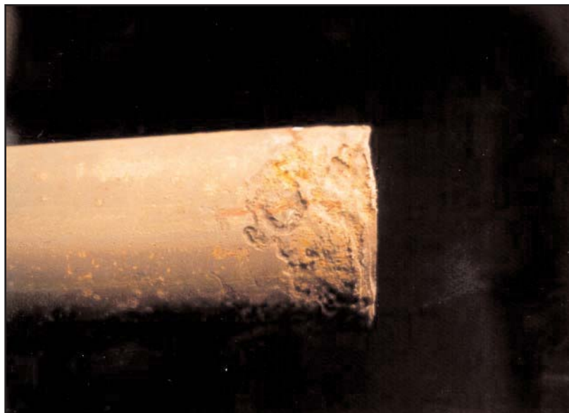
Figure IX-1: Localized Metal Loss at End of Tube that Contacted Bottom Tubesheet
