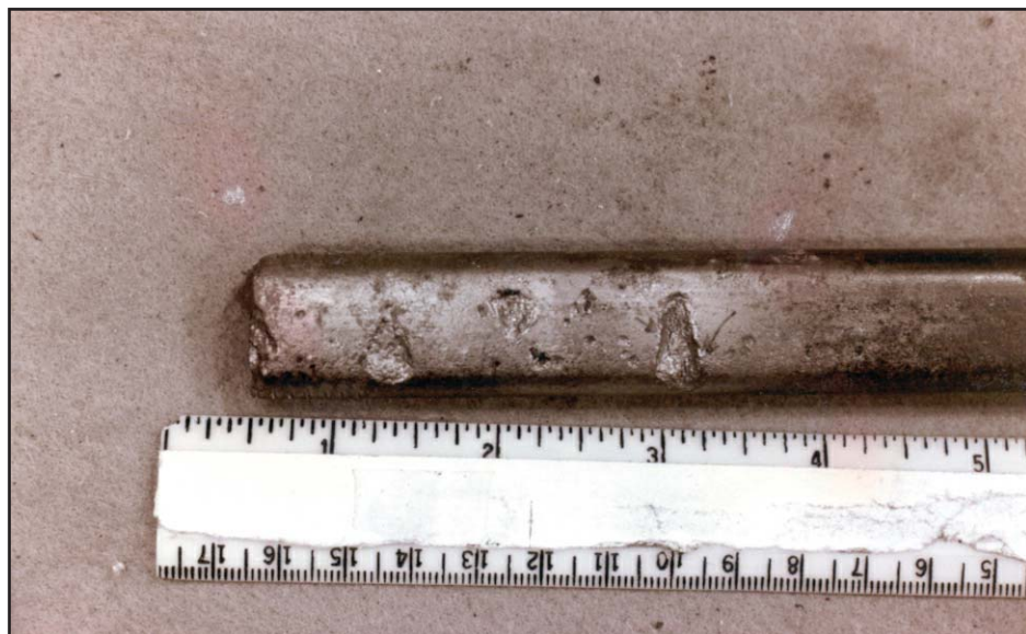
Figure III-5: H 2 S Attack on Sucker Rods Followed by Corrosion Fatigue Break
