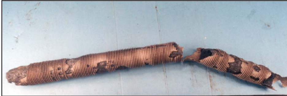
Figure VII-1: De-alloying Tubes — H 2 S Corrosion 90-10 Cu:Ni Heat Exchanger Tubes
