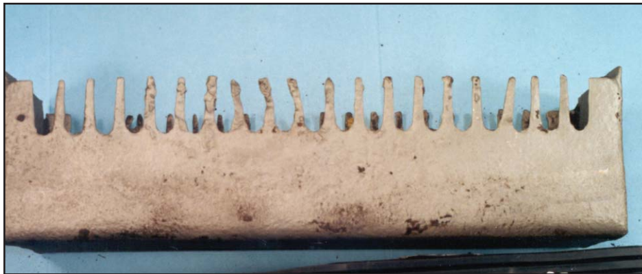
Figure V-12: Underdeposit Corrosion — Note the thinning cleaned surface
