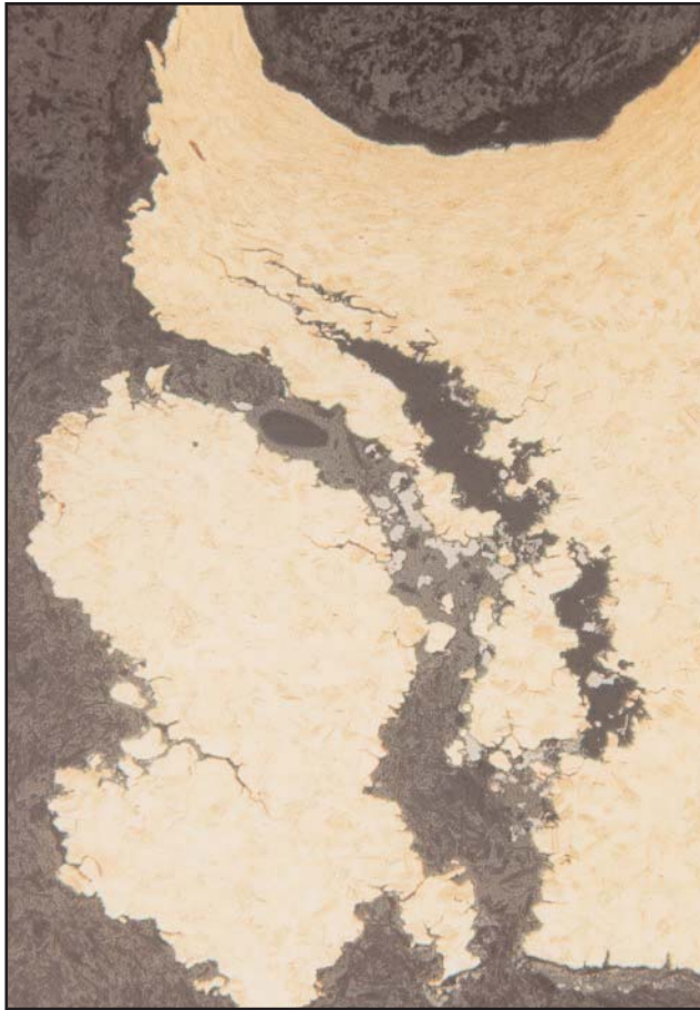
Figure IX-28: Branched, Intergranular Crack and Fissures Penetrating from Internal Surface
