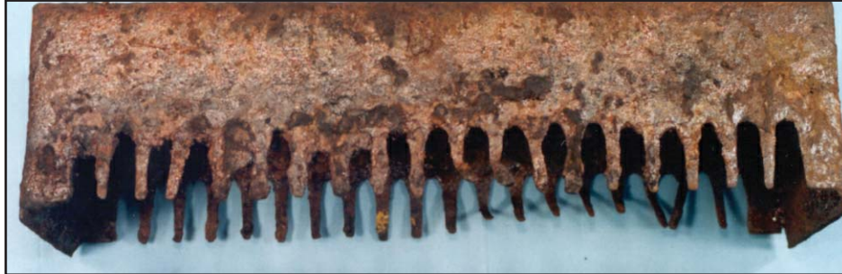
Figure V-11: Carbon Steel Trays — HCl Corrosion
