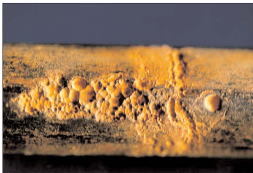
Figure IX-39: Clusters of Mutually-intersecting, Rounded Depressions
