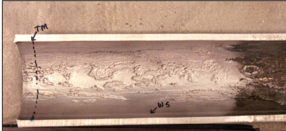
Figure I-29: Mesa Attack on Tubing
