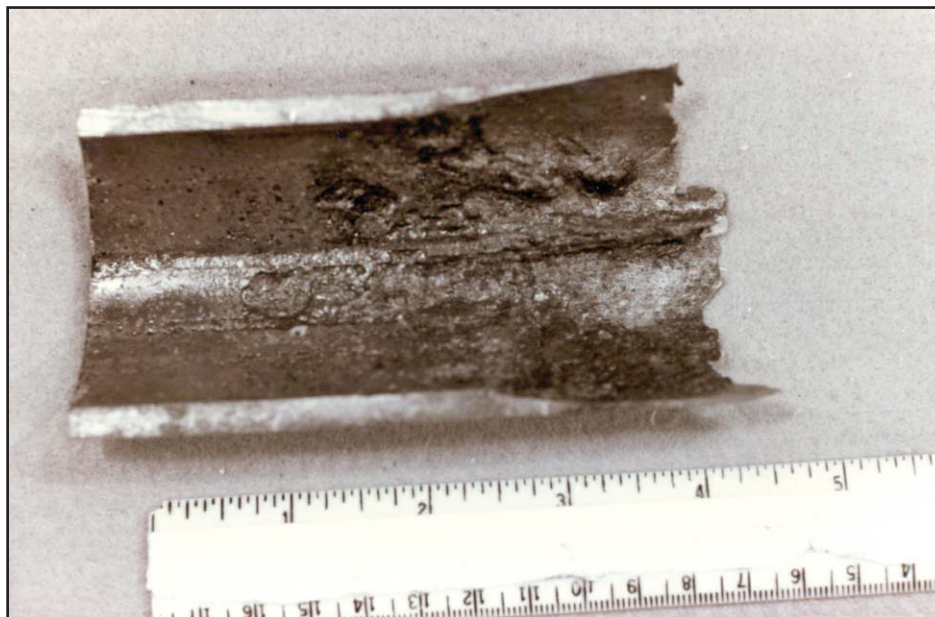
Figure I-20: Severe Thinning Caused by Ringworm Attack
