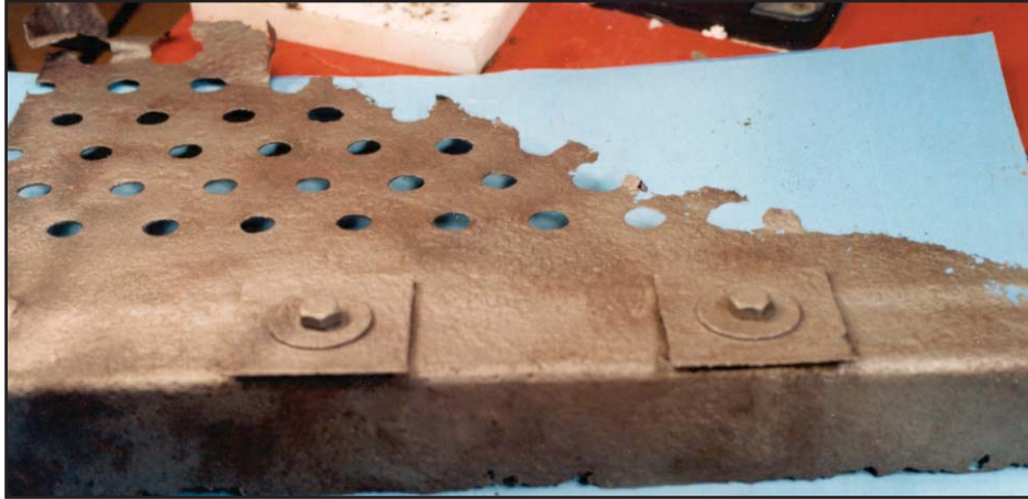
Figure V-13: Sulfidation/Oxidation or Ammonium Chloride
