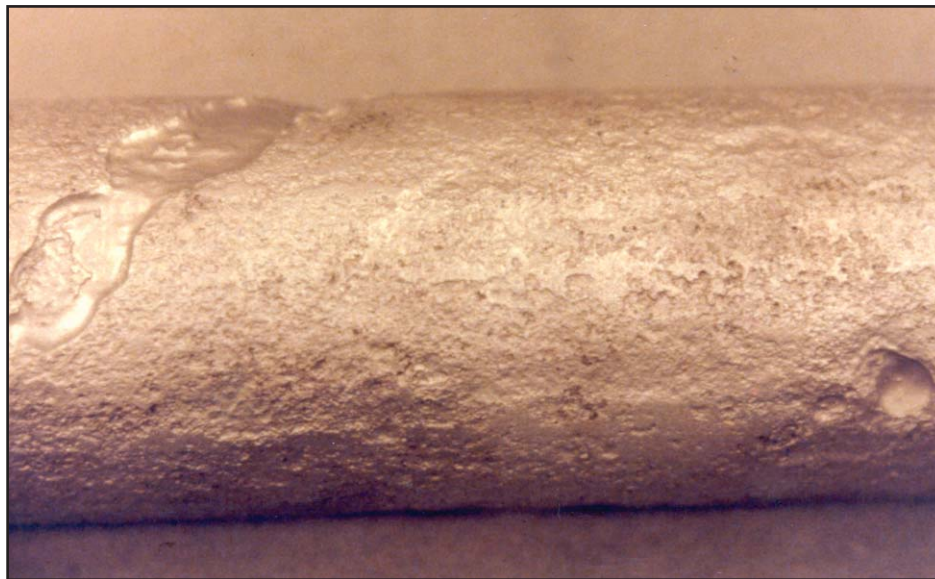
Figure I-27: Corrosion Resulting from Rolled-in Inclusions
