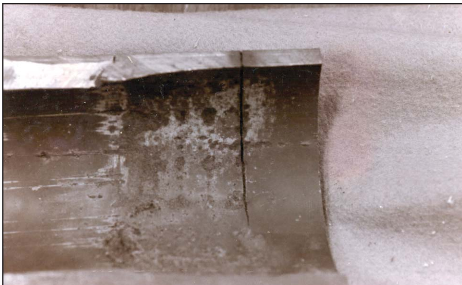
Figure I-52: Corrosion Fatigue in Drill Pipe
